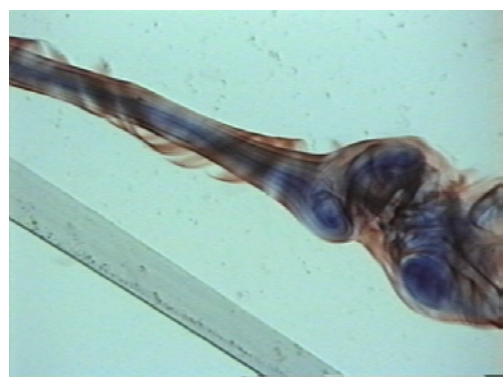
Fig. 5. The apex vortex breakdown (blue) wrapped around by the surrounding flow (red).
