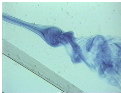
Fig. 4. Zoom-in of the apex vortex breakdown (from the area shown in Fig. 3).
